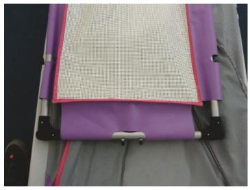
**(N)** Both ends of the top frame should now look like this, with all wing nuts facing outwards and all the spring buttons correctly seated into the plastic fittings.
