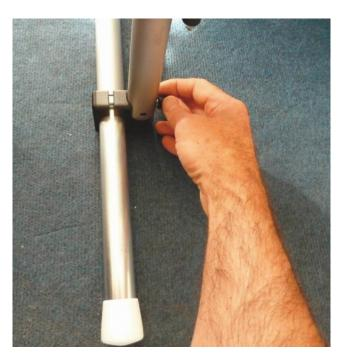
Slide the bar out to increase stability. NOTE: always leave at least 2" inside the outer tube for safety.
